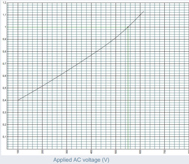
I 2 t multiplier coefficient 550V 4400 to 5000A
